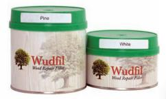
A two part (filler & hardener) filler which can be stained, painted, or varnished. Hardening takes approximately ten minutes after which Wudfil can be easily sanded and sharp edges can be formed without crumbling.
